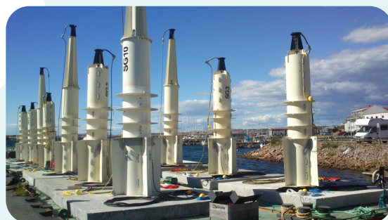
Figure 3 : Dispositif Seabased point absorber
